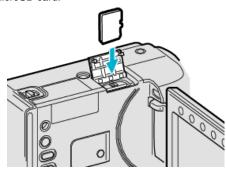
Insert with the metal contact area facing outward.
