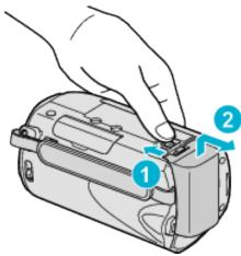
Slide the battery release lever to detach the battery from this unit.
