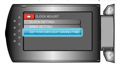
${\it 4}~$  Set daylight saving time with the +/- button and press OK.
