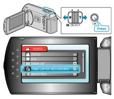
3 Select a recording interval (1 to 80 seconds) and press OK.
