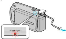
The charging lamp blinks when charging is in progress.
