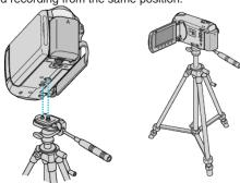
To prevent this unit from falling off, check the tripod mounting screw holes and positioning holes on the unit carefully before mounting, and turn the screws until they are fastened firmly.
