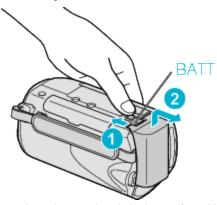
Slide the battery release lever to detach the battery from this unit.
