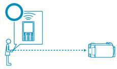
• Any obstacles or human subjects between the Bluetooth-compliant device and the camcorder will interrupt the communication.
