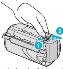
Slide the battery release lever to detach the battery from this unit.
