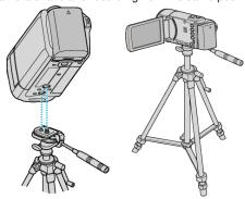
To prevent this unit from falling off, check the tripod mounting screw holes and positioning holes on the unit carefully before mounting, and turn the screws until they are fastened firmly.
