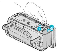
Slide the battery release lever to detach the battery from this unit.
