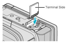
• Insert with the terminal side facing outward.
