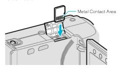
• Insert with the metal contact area facing outward.
