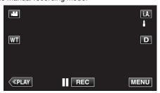
If the mode is i.A. Intelligent Auto, tap i.A. on the recording screen to display the mode switching screen.
