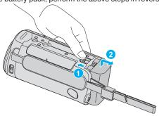
Slide the battery release lever to detach the battery from this unit.
