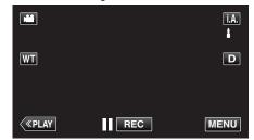
If the mode is i.A. Intelligent Auto, tap i.A. on the recording screen to display the mode switching screen.
