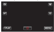
If the mode is M Manual, tap M on the recording screen to display the mode switching screen.
