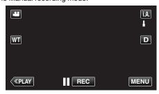
If the mode is i.A. Intelligent Auto, tap i.A. on the recording screen to display the mode switching screen.
