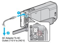
• The charging lamp blinks when charging is in progress. It goes out when charging is finished.
