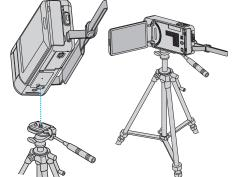
To prevent this unit from falling off, check the tripod mounting screw holes and positioning holes on the unit carefully before mounting, and turn the screws until they are fastened firmly.
