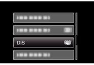
3 Select "ON" or "ON (AIS)" to activate the image stabilizer and press OK.
