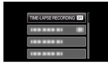
3 Select a recording interval (1 to 80 seconds) and press OK.
