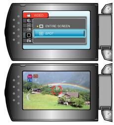
When "SPOT" is selected, select the position of the spot frame by pressing the +/- buttons.
