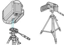
• To prevent this unit from falling off, check the tripod mounting screw holes and positioning holes on the unit carefully before mounting, and turn the screws until they are fastened firmly.
