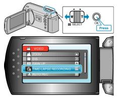
${\it 3}$  Select a recording interval (1 to 80 seconds) and press OK.
