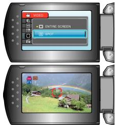
When "SPOT" is selected, select the position of the spot frame by pressing the +/- buttons. After selecting, press OK to confirm.
