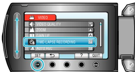
4 Select a recording interval (1 to 80 seconds) and touch **OK**.
