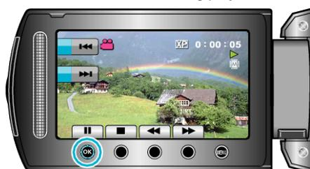
• After pausing the video, you can fine-tune the point to capture by using the forward slow-motion  $\blacktriangleright$  and reverse slow-motion  $\blacktriangleleft$  operation buttons.
