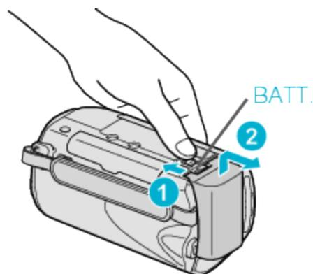
Slide the battery release lever to detach the battery from this unit.
