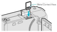
• Insert with the metal contact area facing outward.
