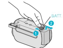
Slide the battery release lever to detach the battery from this unit.
