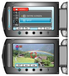
When "SPOT" is selected, select the position of the spot frame by touching the operation buttons "←"/"→".
