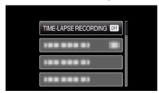
3 Select a recording interval (1 to 80 seconds) and press OK.
