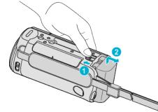
Slide the battery release lever to detach the battery from this unit.
