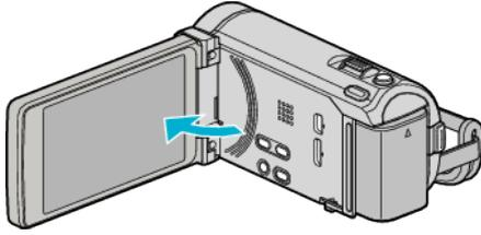
2 Connect the USB cable and the AC adapter.
