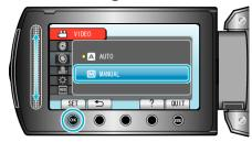
5 Adjust the focus with the slider.
