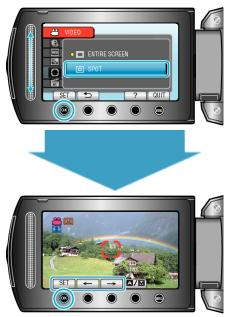
When "SPOT" is selected, select the position of the spot frame by touching the operation buttons "←"/"→".
