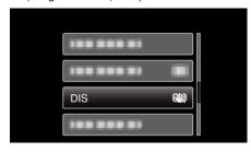
3 Select "ON" or "ON (AIS)" to activate the image stabilizer and press OK.
