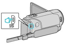
• Press the "START/STOP" button to start a normal recording.
