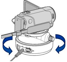
• When the power is turned ON, pan cradle moves to the left/right to adjust the position.
