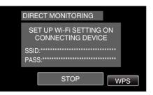
6 Select the SSID in step 5 from the Wi-Fi network selection screen of your smartphone, and enter the PASS on the password screen. (Operation on the smartphone (or computer))
