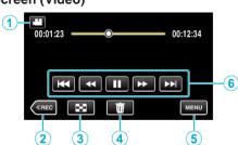
• Operations buttons on the touch screen disappear if the unit is not operated for about 5 seconds. Tap on the screen to display the operation buttons again.
