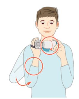
Hold the LCD monitor with your left hand and adjust the angle accordingly. Holding the LCD monitor with your left hand helps to stabilize the camera for recording.
