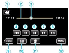
• Operations buttons on the touch screen disappear if the unit is not operated for about 5 seconds. Tap on the screen to display the operation buttons again.
