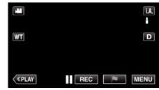
If the mode is **i**.**A**. Intelligent Auto, tap **i**.**A**. on the recording screen to display the mode switching screen. Tap M to switch the recording mode to Manual.
