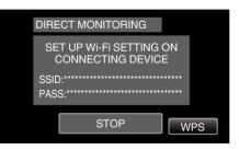
6 Select the SSID in step 5 from the Wi-Fi network selection screen of your smartphone, and enter the PASS on the password screen. (Operation on the smartphone (or computer))
