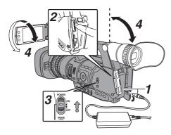
1 Supply battery or AC adapter power to the camera recorder.
