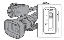
When the camera recorder is in the Scene Select mode, "SCN A" or "SCN B" appears on the screen.
