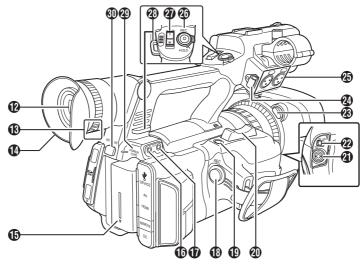
(B) [REC] Record Trigger Button Starts/stops recording.
