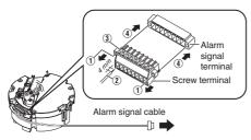
① Loosen screws on both sides of the screw terminal with a flathead screwdriver, and remove the screw terminal.
