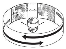
Specifies the auto pan settings. This item sets the Auto Pan operation which moves at a specific speed from the preset [Start].
