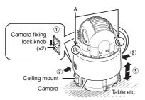
Release the locks by sliding them in the direction indicated by the arrows (2) Push the lock knobs inward from both the left and right directions as indicated by the two arrows.
